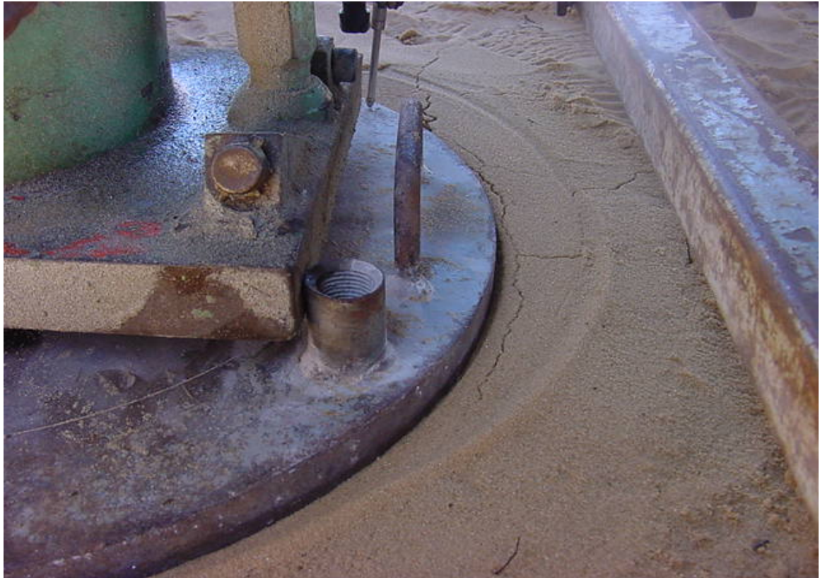
Figure C.5: A photo shows a radial failure occurred while performing load plate test on the sandy soil on site around plate of 45 cm diameter
