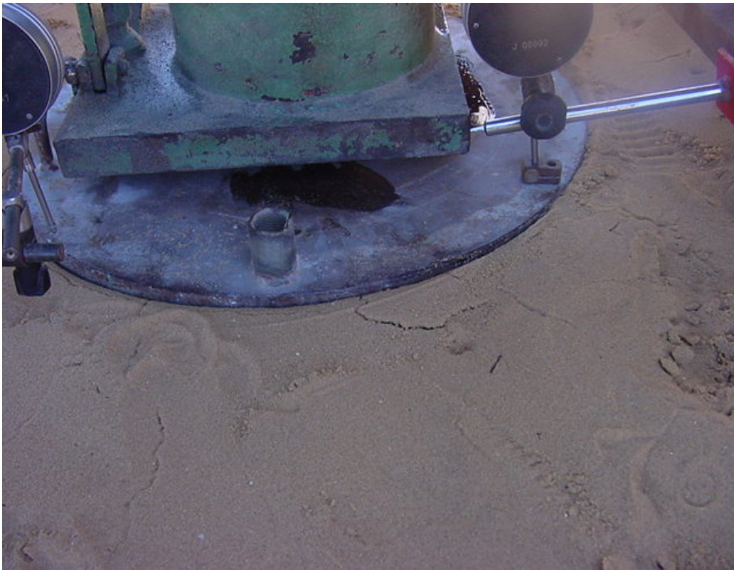
Figure C.2: A photo depicts the shape of failure seen on site in the sandy soil
