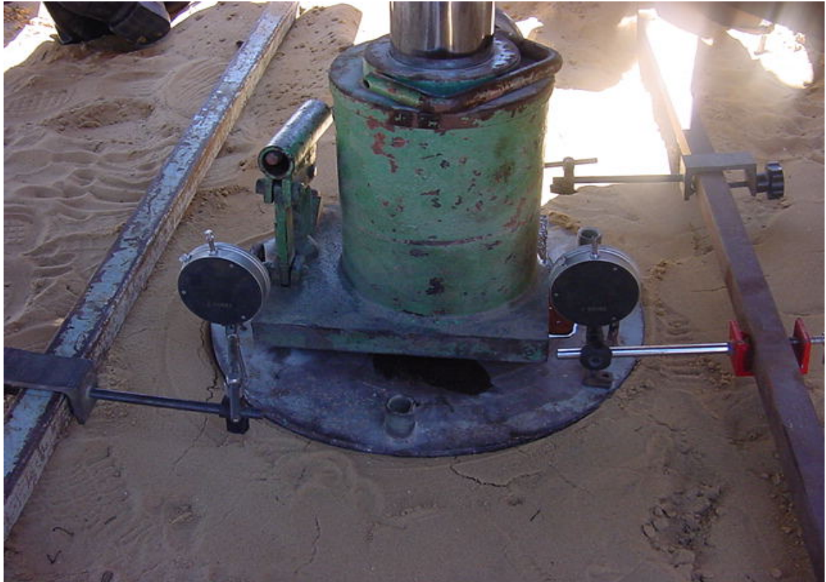
Figure C.3: A photo shows the load cell, strain gauges and the reference beams
