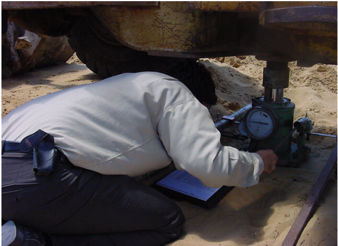
Figure C.6: A photo shows the adjustment plate load and strain gauges in field
